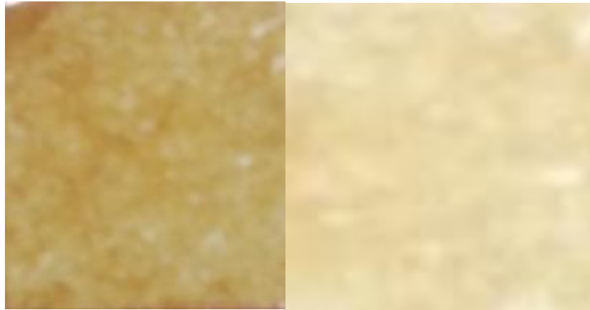
Figure 1. Samples of marble coated by cod liver oil
