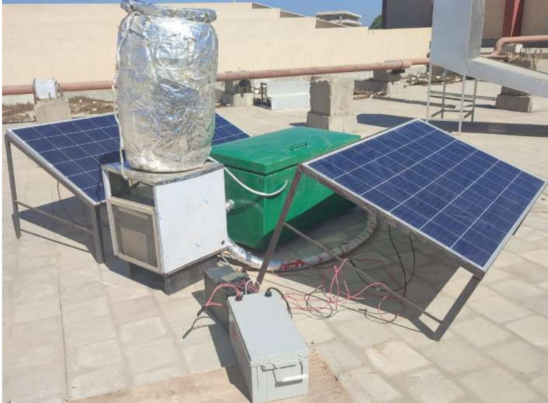
Fig. (1): The developed solar chiller for tomatoes pre-cooling
